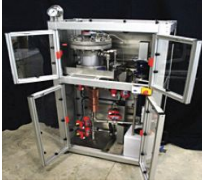
Figure 3.3 “Loughborough University has developed a user-friendly, fully operational household toilet system that transforms feces into biochar through the hydrothermal carbonization of fecal sludge.” Source: Gates Foundation, n.d.
